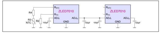
In Figure 5.2, note that each ZLED7010 can drive up to three slave ICs in the next stage. Using more than three stages to maintain current coherence is not recommended. Up to thirteen ZLED7010 can be connected in one system.
